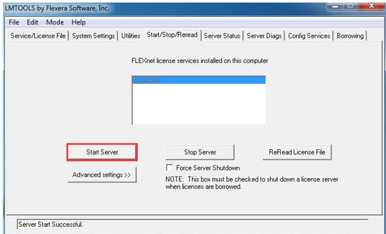
You can start server either manually or automatically, it is to select Start/Stop/Reread option to control the server in Start/Stop/Reread tab or control sever automatically in Config Services tab by checking User Services and Start Server at Power Up when start the computer.
