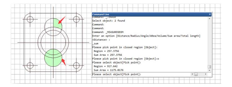
Total length: Calculates the object length and total length associated with selected arc, circle, polyline segments or line objects. you can either select the single object by click or select multiple objects with window selection.
