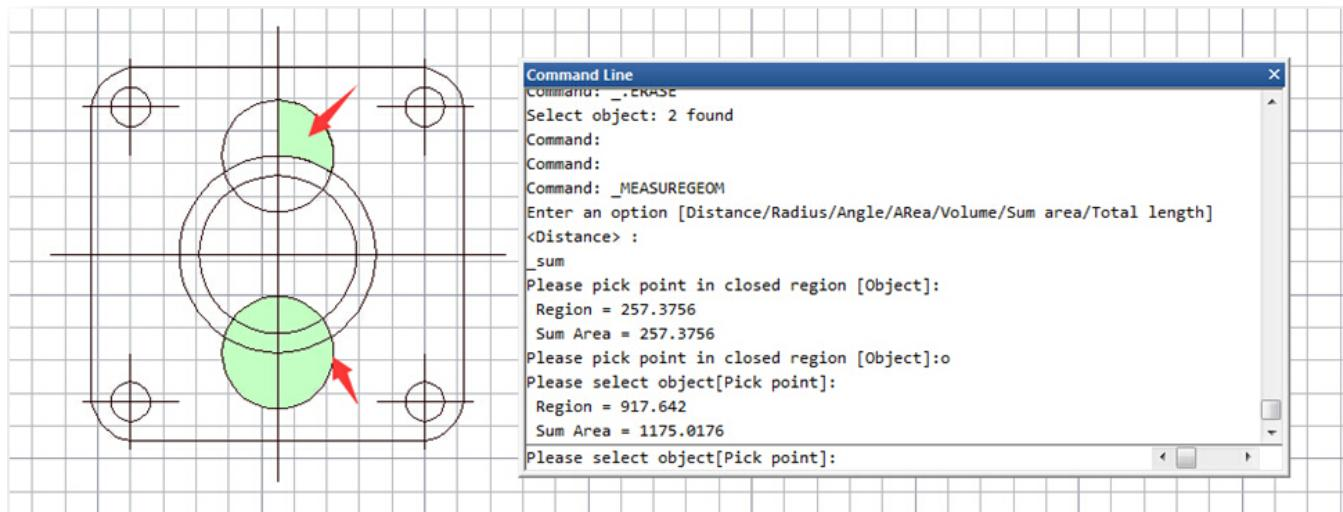
Total length: Calculates the object length and total length associated with selected arc, circle, polyline segments or line objects. you can either select the single object by click or select multiple objects with window selection.
