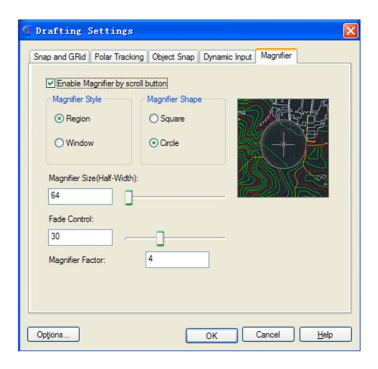
Enable Magnifier by Scroll button:If you check this option you can enable/disable the magnifier command by clicking the scroll wheel of the mouse. Also the shortcut key Ctrl+E is available to activate magnifier.
