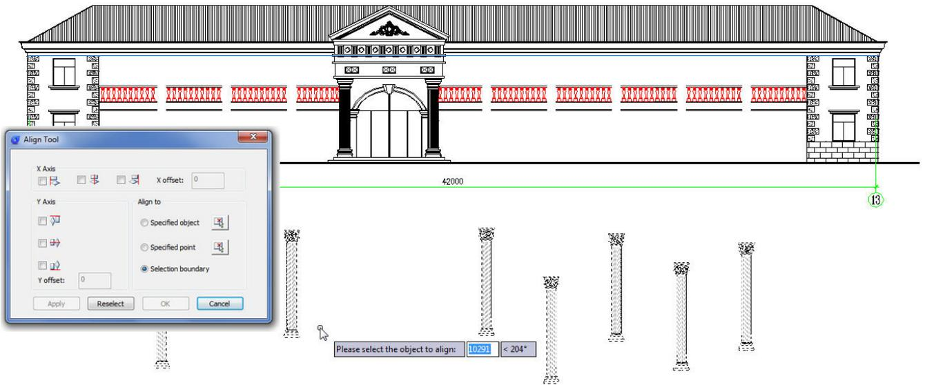
After you have selected the objects, the Align tool settings window will pop up: first we have to check the option Top object under Y axis alignment. After check this option the objects (columns) will be aligned at same level:
