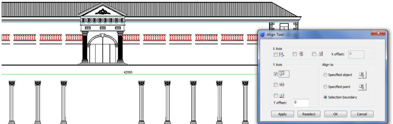
After the objects have been aligned, we have to select the option specified object under Align to. Then select the object (blue line) where we want to align and place the objects. Finally you will get a faster result performing this operation:
