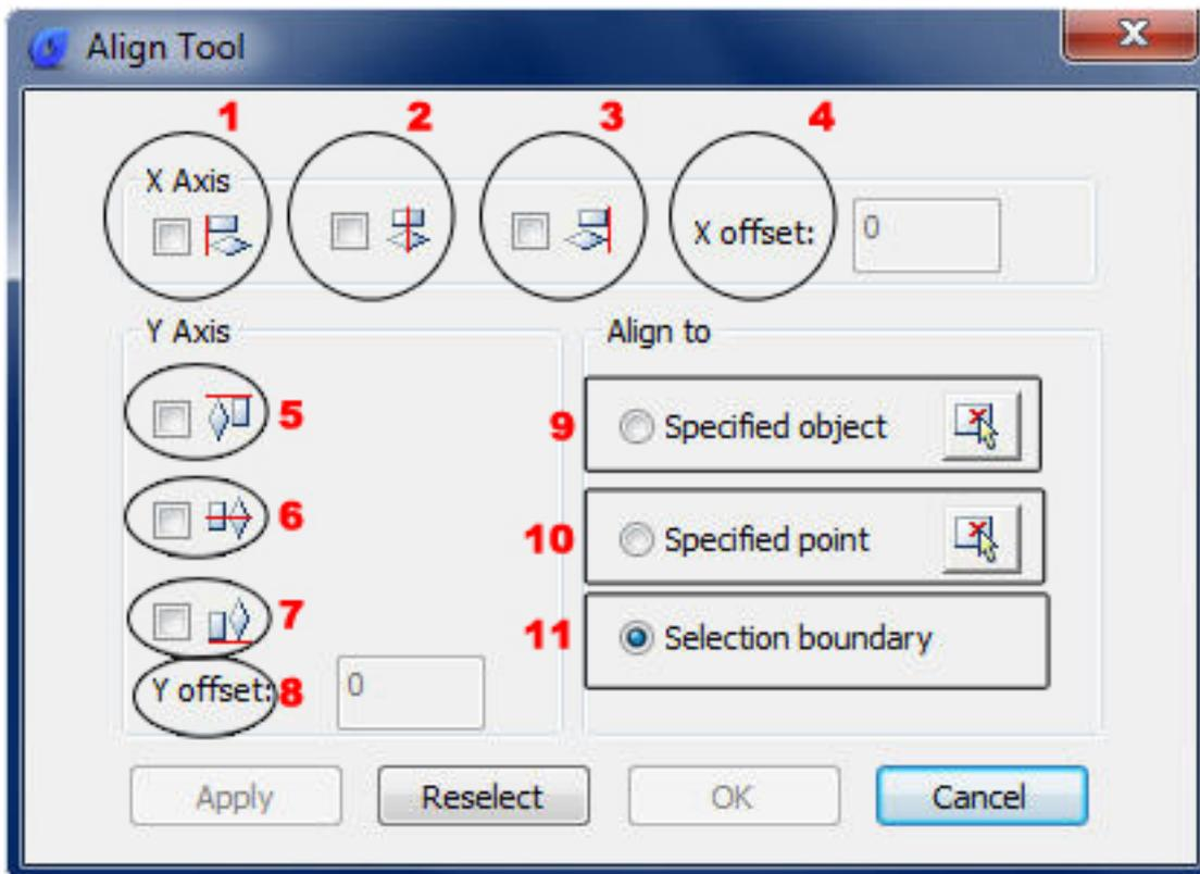
1.- Left object X axis Align: This allows to align the selected object(s) at the left side according to the X axis.
