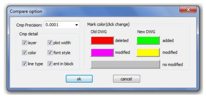
After setting up the comparison parameters such as: colors, layers, line type, etc. select Ok to confirm these parameters. Note: Pay attention to the mark color because the deleted, modified and added objects will assume these into the compared drawing. Then select the button Compare in the window below to compare both drawings.
