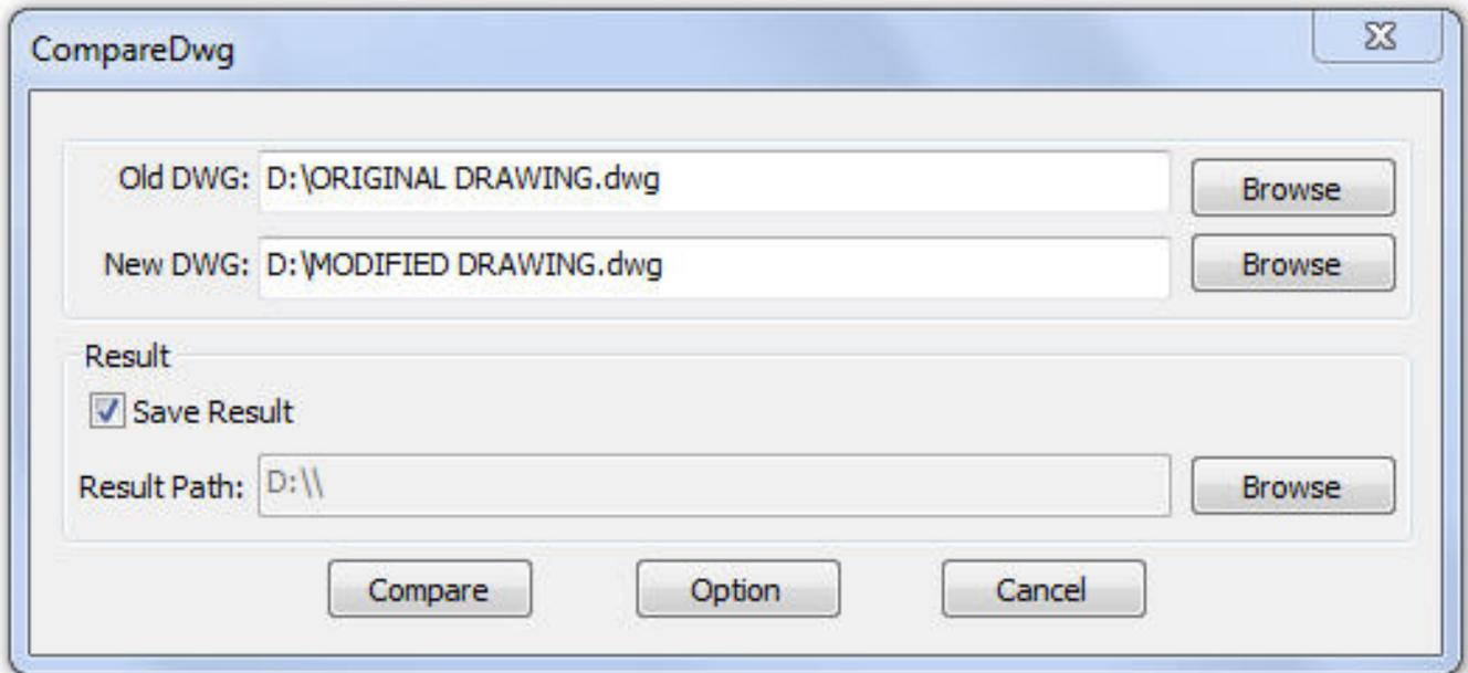
In this window, you have to browse the old DWG (original drawing) and the new DWG (drawing modified). You can also assign a path to save the compared drawing. Then select the button Option to set-up the comparison parameters.
