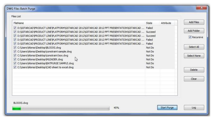
**Log**: After the purge operation is finished, you can Login in to the created notepad file and see the batch purge detail record.
