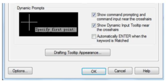
When the dynamic input tooltip is fixed, it turns semi-transparent as default. At this stage you can freely move the cursor over the workspace but when you move it over the dynamic input, it will be highlighted. What's more, you can select a command option with the cursor.
