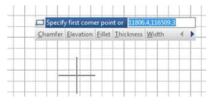
Within Drafting Settings dialog box, under Dynamic Input tab, there is an option called Automatically Enter when the keyword is Matched. This option allows to typing the CAPITAL letter of the command option to be selected. After typed, you don't need to press ENTER. The option will be executed automatically. With this option ,your drafting design efficiency can be enhanced greatly.
