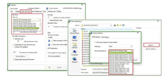
You can access it in option dialog box, in open and save tab, under File Save option. Also, in the Save drawing as dialog box, select options and change the default to the lowest file format the other users can open it. Now you don't have to worry the others can't open your GstarCAD files!
