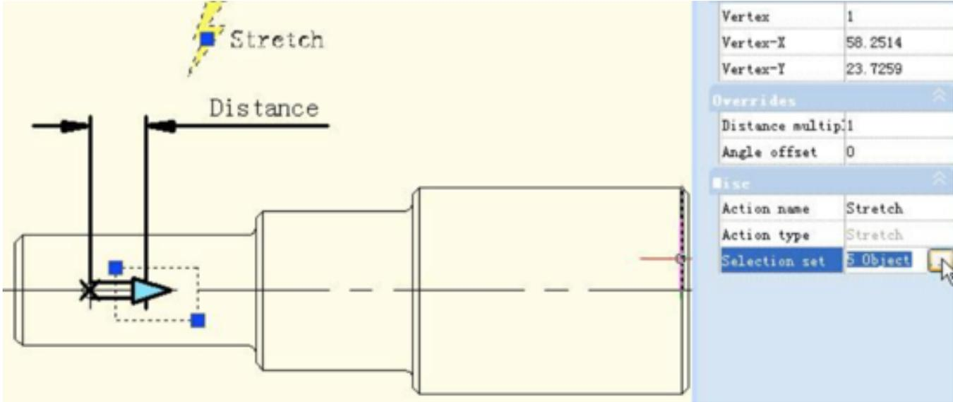
Blacken object is the operational object of the action, broken line frame is the stretch frame, objects intersect with stretch frame will be stretched, objects which be selected by stretch frame will move.
