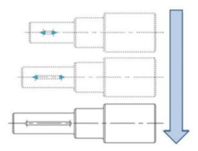
The realization of chain action has two important procedures: First, modify the property value of the parameter that need to happen linkage and modify the property of "chain action" from "NO" to "YES". Second, select the parameter of objects that selected to linkage action to set.
