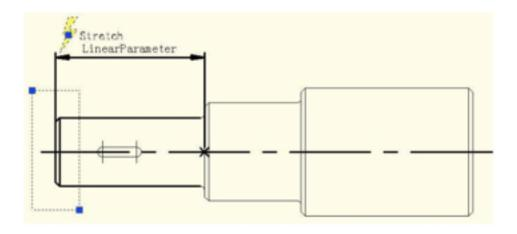
Because the follow-up operation will not stretch step shaft by grips of this linear parameter, the grip"s number of linear parameter can be modified as "0".
