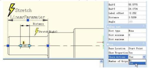
Add Stretch Leftwards action for keyway as the following picture shows. Special Notes: Do elect "Distance" to
