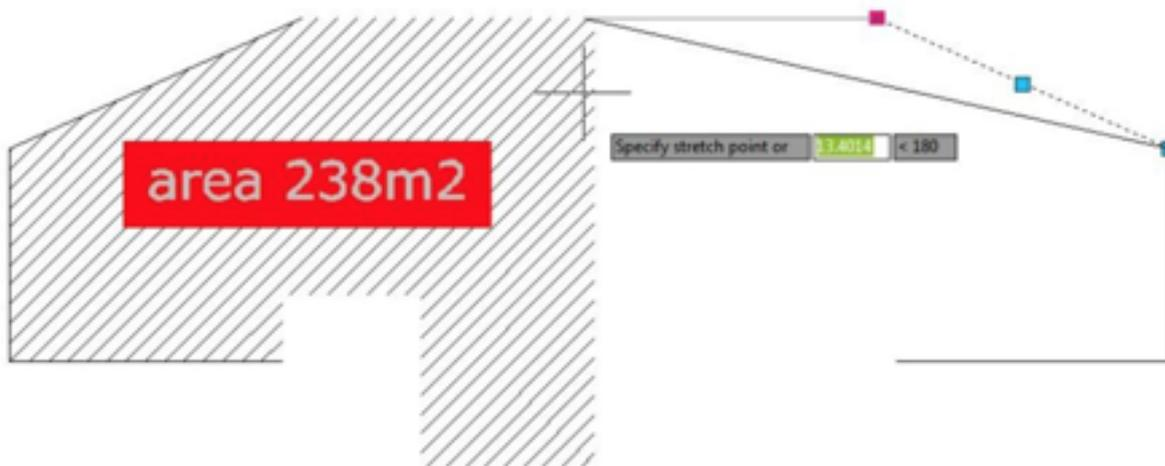
To activate it, simply issue OPTION command. In option dialog box, drafting tab, in object snap options, turn off ignore hatch objects. You can also set this option by changing OSOPTIONS system variable.
