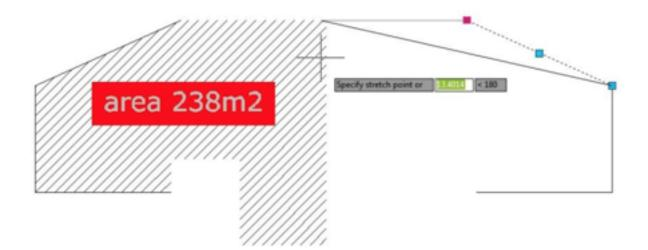
To activate it, simply issue OPTION command. In option dialog box, drafting tab, in object snap options, turn off ignore hatch objects. You can also set this option by changing OSOPTIONS system variable.
