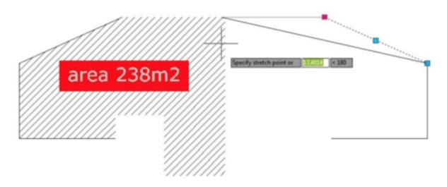
To activate it, simply issue OPTION command. In option dialog box, drafting tab, in object snap options, turn off ignore hatch objects. You can also set this option by changing OSOPTIONS system variable.
