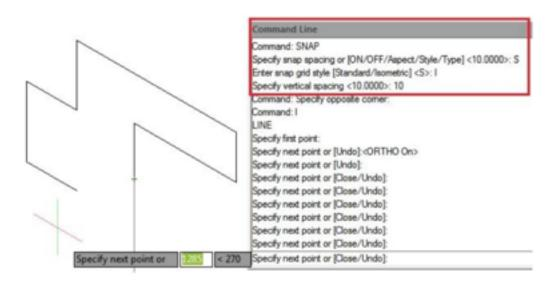
Also you can change your plane by typing ISOPLANE [enter] then select left, top, right.Alternatively, you can use the SNAPSTYL command, changing the variable value to 1. You can change your plane by typing ISOPLANE, but it can be done faster by pressing "F5" key. To came back to the default, use the SNAPSTYL command again and change the variable value to 0.
