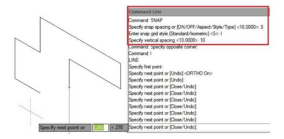
Also you can change your plane by typing ISOPLANE [enter] then select left, top, right.Alternatively, you can use the SNAPSTYL command, changing the variable value to 1. You can change your plane by typing ISOPLANE, but it can be done faster by pressing "F5" key. To came back to the default, use the SNAPSTYL command again and change the variable value to 0.
