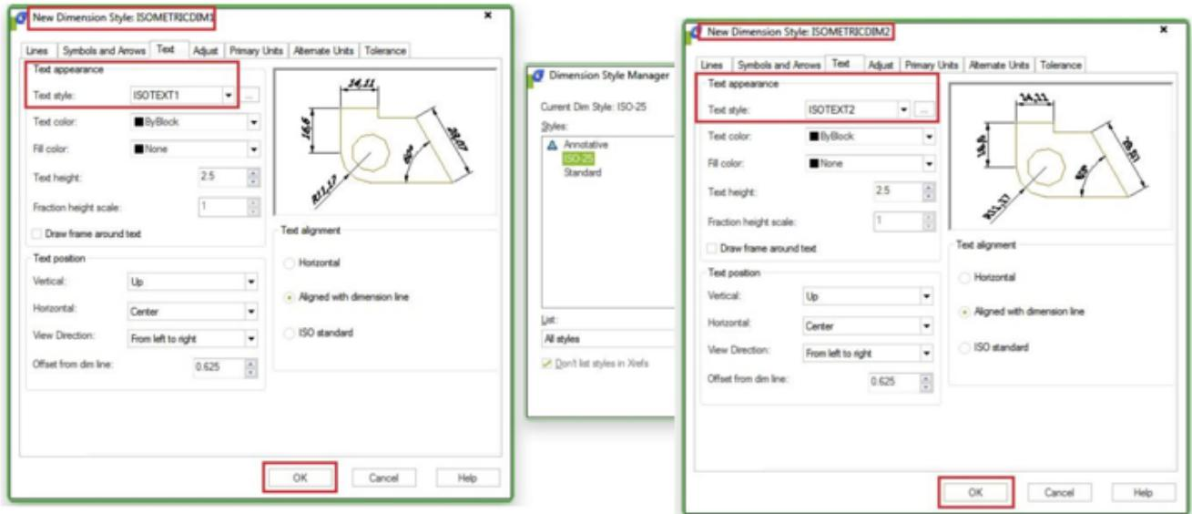
Now place aligned dimension. Notice that the extension lines of the dimension placed are not perpendicular as the blue line. Now we have to do a little modification.
