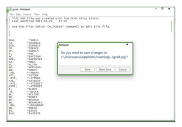
As you can see, the list of all GstarCAD command aliases by default. So aliases for line is L. When I type L then [enter] will activate the line tool. Typing LA [enter] will open the layer manager. Etc. They are very useful shortcuts to work faster! You can edit the command aliases and change them to what you want. After you finish, save this file. You might need to restart your GstarCAD after doing your modification. Or you can run REINIT to reload your gcad.pgp.
