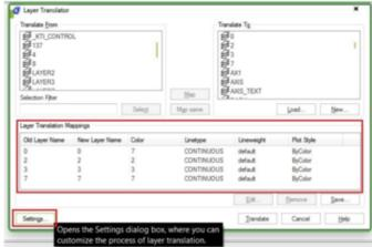
With the layer translator settings, you can setup layer properties to be translated into the assigned layer of your drawing standards that you need.
