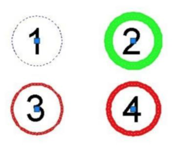
Only block no.2 using the block properties, because we set it the geometry properties to by block. Now freeze Layer1. We can see the block no. 4 disappeared, because the object in it was created on it.
