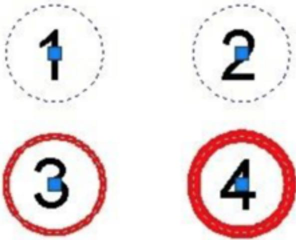
3. Now override the color and line weight. Use color green, and line weight 2. You can see that the only block using the overridden properties is block no. 2!
