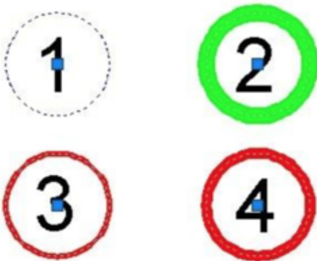
Only block no.2 using the block properties, because we set it the geometry properties to by block. Now freeze Layer1. We can see the block no. 4 disappeared, because the object in it was created on it.
