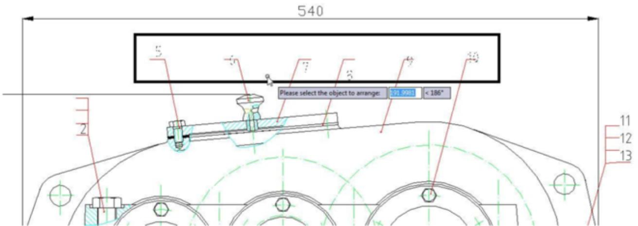
Then select the part numbers. After select the part numbers, the arrange tool window will pop up, select the option: Specify spacing and then check or select the option: Top vertical arrangement. See the result below:
