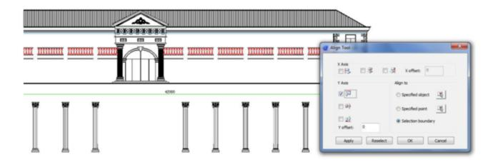
After the objects have been aligned, we have to select the option specified object under Align to. Then select the object (blue line) where we want to align and place the objects. Finally you will get a faster result performing this operation:
