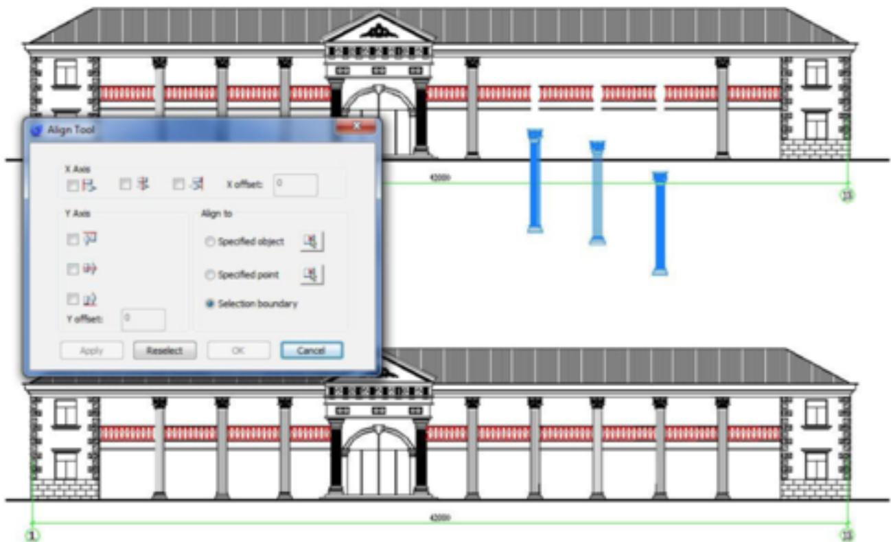
As an example, we will put this tool in action. We can apply this tool to align a high quantity of objects (columns) in the correct place in this complex drawing as shown in the picture below:
