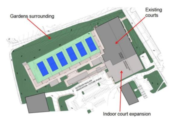
After started the command, you have to pick an internal point(s) in the closed region(s) to see the area result. For example, if you want to know the area sum of existing courts including the indoor court expansion, just pick and internal point of each closed objet. After picking points, the command line will show up in real time the region value sequence and area sum in (mm2):
