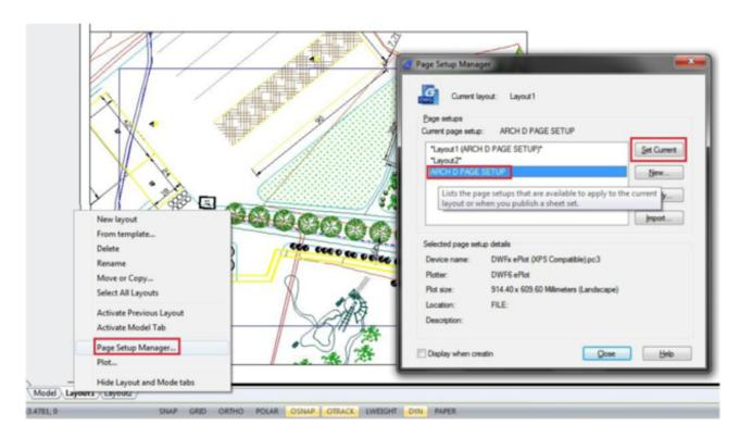
Not only do Named Page Setups saved you time configuring each layout tab to plot correctly; they prevent Sheet 1 plotting different from Sheet 2 because someone accidentally assigned the ARCH D (36.00 x 24.00 Inches) page size to one sheet and the ARCH expand D (36.00 x 24.00 Inches) to the other. For such a small feature, the standardization benefits can be far-reaching.
