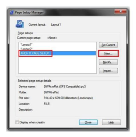
Below you can see, I"ve configured a Named Page Setup that uses the DWFx ePlot plotter, an ARCH expand D page size, and the gcad.ctb plot style table. Instead of manually changing these on each of my drawing sheets (Layout tabs).
