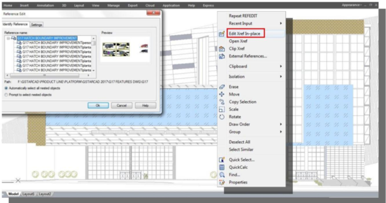
The objects that you select from the selected xref or block are temporarily extracted and made available for editing in the current drawing. The set of extracted objects is called the working set, which can be modified and then saved back to update the xref or block definition.
