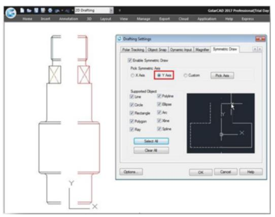
**Custom/Pick Axis option**: The objects drawn will take the vector orientation of a selected object as visible axis line. The effect of Custom/Pick Axis is mirroring the drawn objects according to a selected object vector orientation whether inclined, vertical or horizontal.
