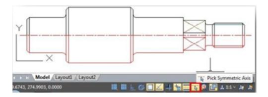
Technical Demo - Symmetric Draw is an innovative tool to directly draw symmetrical shapes. When drawing the first half you get another half automatically.
