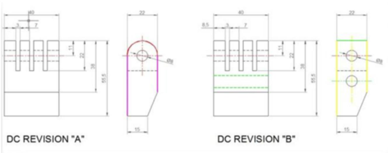
So the details are very important when comparing objects. Now the new and innovative Graphic Compare tool can do more! It does not only compare two drawings with similar objects geometry and find out the differences but also display the details of any change at the current workspace of your drawing in real time, e.g. if a line is modified, only the changed part of the line is displayed in different color. The unchanged part remains unchanged.
