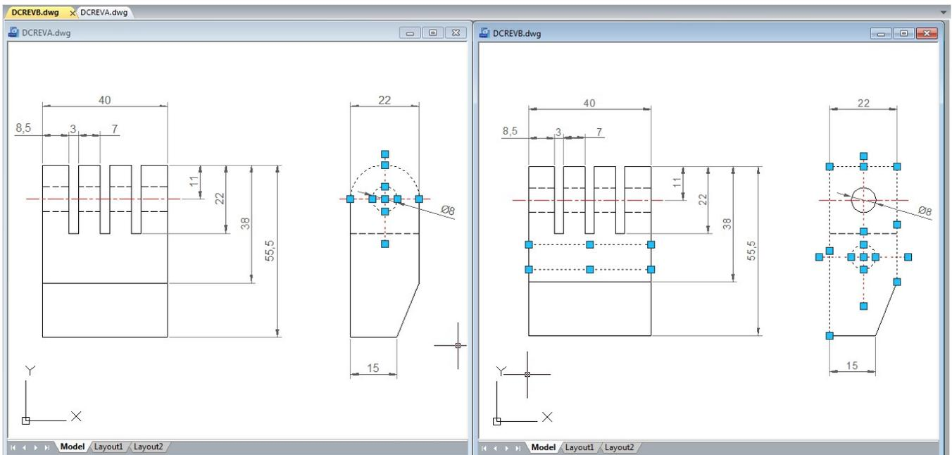
Drawing compare can make comparisons between two similar drawings (old DWG and New DWG) and generate them as separate files. After pressing COMPARE button within CompareDwg dialog box, the program will generate and open \_old and \_new.dwg files, where you can see the differences between drawings.
