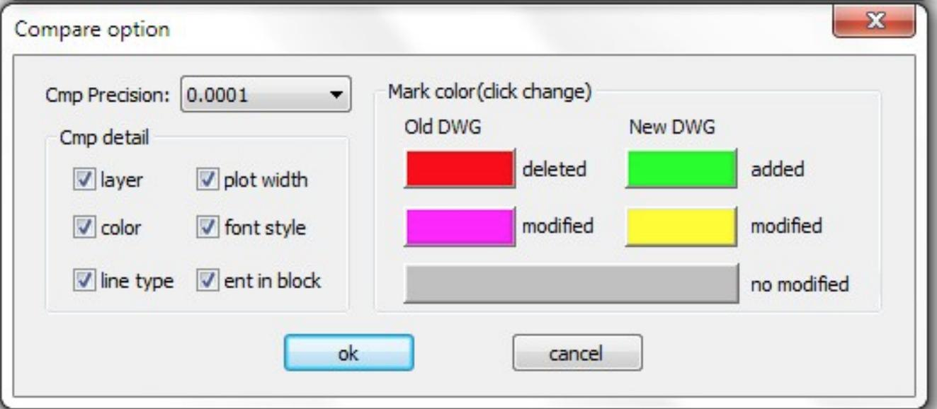
Drawing Compare can find out differences (drawn objects) and show the result with different colors, e.g. if a line is modified, removed or newly drawn, it will be displayed in different colors.
