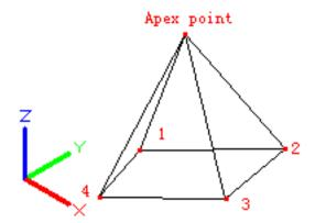
• **Ridge:** Define the top of pyramid as a ridge. The order of two endpoints should be the same as base points to avoid self-intersection.
