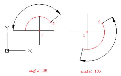
• **Chord length**: Create an arc by a specified chord length; the chord is a line segment from the start point to endpoint of arc. If specifying the chord length to a positive value, it will create a minor arc from the start point in anticlockwise direction; if specifying a negative value, it will create a major arc in anticlockwise direction.
