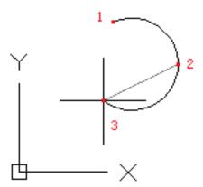
Those three points could specify an arc clockwise or anticlockwise.
