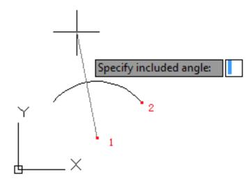
• Chord length: The point 1 is center of arc. The chord length is the distance from the point 2 to the endpoint. Users could create a major arc or minor arc by specied chord length. If inputting a positive chord length value, it will create a minor arc in anticlockwise; if inputting a negative chord length value, it will create a major arc in anticlockwise.
