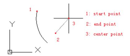
• Angle: Create an arc with a specified angle from start point to endpoint. If the inputted angle is negative, the arc will be created in clockwise direction.
