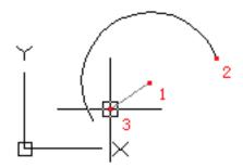
• **Angle**: Specify the center 1 and create an arc from the start point 2 with a specified included angle. If the included angle is negative, the arc will be created in clockwise; if it is positive, the arc will be created in anticlockwise.
