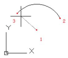
• Angle: The point 1 is center of arc. The included angle is from the point 2. It is created in anticlockwise. If inputting a negative angle, the arc will be created in clockwise direction.
