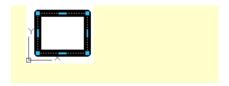
• Add area: In the "Add" mode, it could calculate the total area of defined region. Users could use this option to calculate separate area and circumference of each selected object and calculate the total area of them all.
