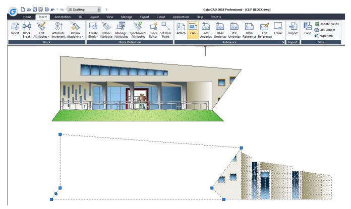
Adjusting the size of the clipped boundary: If you want to change the clip boundary's shape and size of the external reference and block, you can use grips to edit the vertexes just like using grips to edit other objects.
