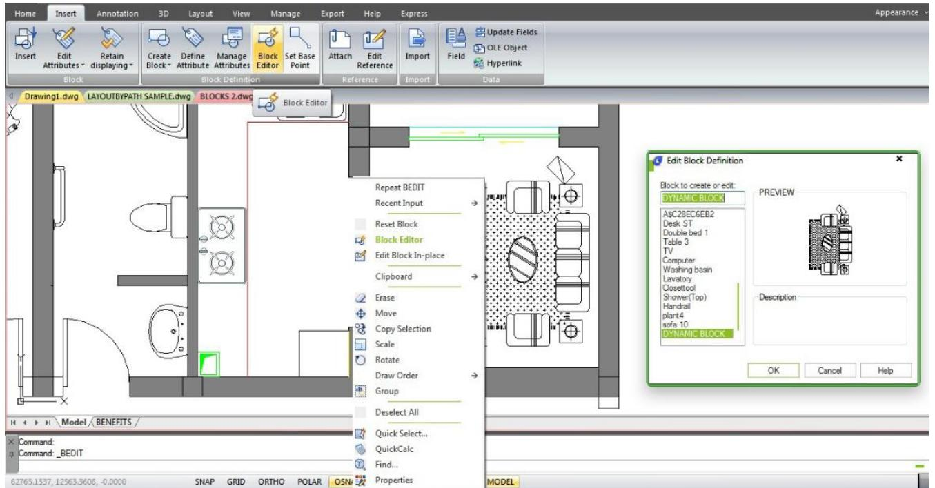
One thing you must remember. When working with block editor, 0,0 is the insertion point. So don't move the geometry unless you want to move the insertion point!
