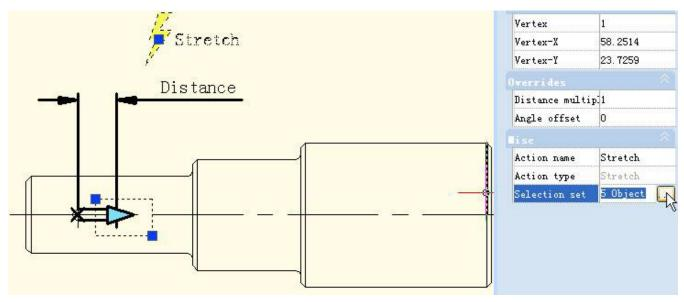
Blacken object is the operational object of the action, broken line frame is the stretch frame, objects intersect with stretch frame will be stretched, objects which be selected by stretch frame will move.
