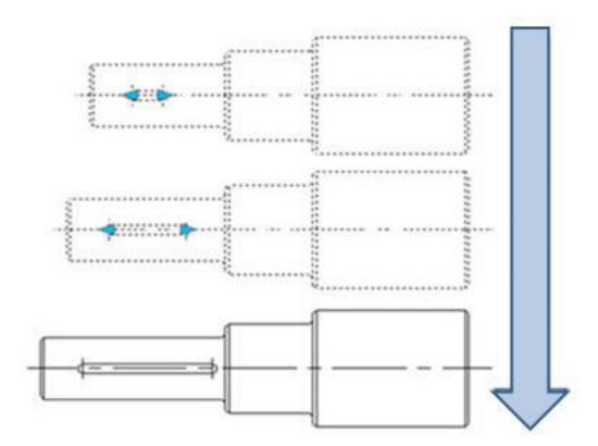
The realization of chain action has two important procedures: First, modify the property value of the parameter that needs to happen linkage and modify the property of "chain action" from "NO" to "YES". Second, select the parameter of objects that selected to linkage action to set.
