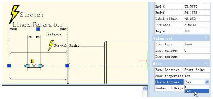
Add Stretch Leftwards action for keyway as the following picture shows. Special Notes: Do elect "Distance" to the linear parameter to stretch leftwards operation objects set. This is a necessary procedure for chain operation.
