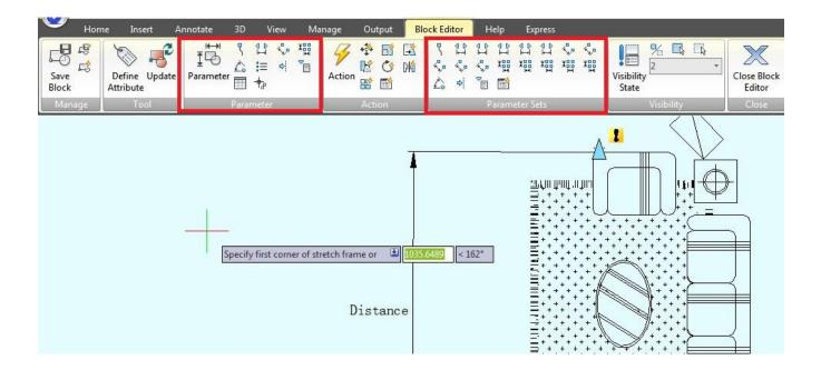
**Point Parameter**: Defines an X and Y location in the drawing. A point parameter can be associated with a move or stretch action.
