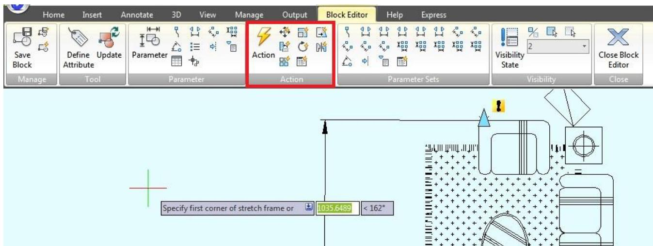
**Move:** Move action causes objects to move a specified distance and angle such as a point, a linear, a polar, an XY parameter, etc, moves all objects in a selection set in a/any direction.
