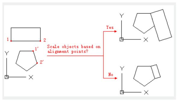
The first source point aligns to the first destination point; the second pair of points defines the rotation angle. It will prompt to scale objects after inputting the second pair of points. The distance from the first destination point to the second destination point is the reference of scale length; it could be used only in two pairs of points.
