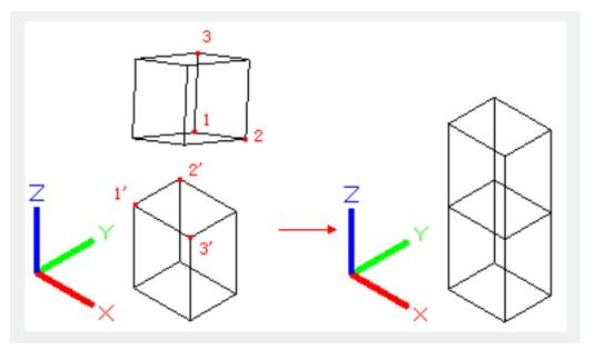
The selected object moves from the first source point (1) to the first destination point (1'); The selected object rotates to align the second source point (2) to the second destination point (2').
