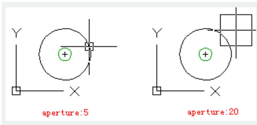
The APERTURE command could control object Aperture box rather than Pick box that displayed under the command prompt of “select object”.
