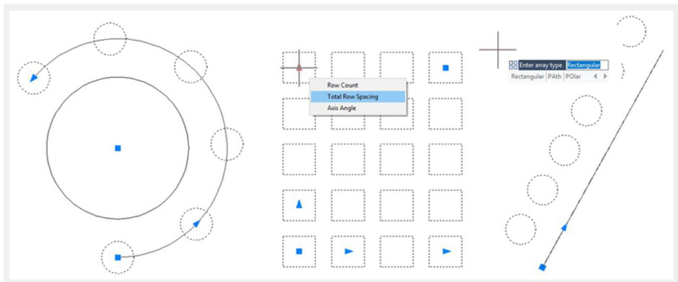
Each element in an array is called array project, which can contain multiple objects. You can also specify blocks as source objects for arrays. If you choose the path array, you also need a straight line, a polyline, a three-dimensional polyline, a spline, a helix, an arc, a circle, or an ellipse to use as a path. For different array types, the Ribbon panel provides different parameter setting options.
