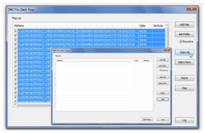
Start Purge: Starts purging the selected DWG file list and it shows a status bar during the execution. After purging, GstarCAD will generate a notepad file where you can see the purge details.
