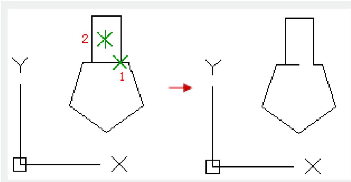
To break an object without deleting one part, users could specify the second point the same as the first point, or input the coordinate of the second point with @. There are many objects could be broken into two parts or removed one of them, such as straight line, arc, circle, polyline, ellipse, spline, torus and others. Taking a circle for example, it could be broken from the first point to the second point in anticlockwise direction, and turns it to an arc.
