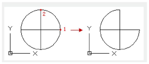
Users could also break an object at a point by the "BREAK AT POINT" tool. This command could break straight line, open polyline and arc except closed objects (such as circle).
