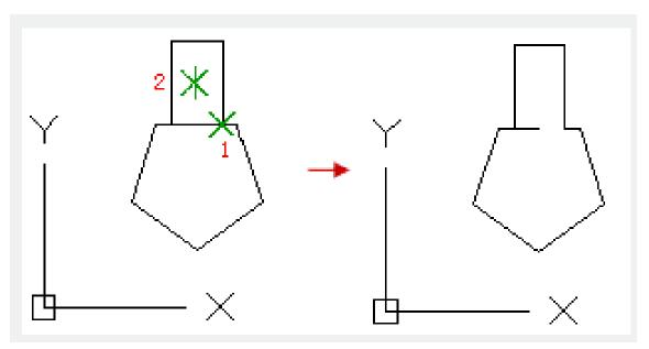
To break an object without deleting one part, users could specify the second point the same as the first point, or input the coordinate of the second point with @. There are many objects could be broken into two parts or removed one of them, such as straight line, arc, circle, polyline, ellipse, spline, torus and others. Taking a circle for example, it could be broken from the first point to the second point in anticlockwise direction, and turns it to an arc.
