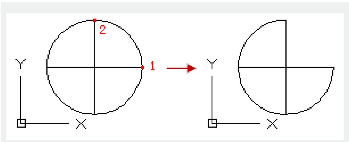
Users could also break an object at a point by the "BREAK AT POINT" tool. This command could break straight line, open polyline and arc except closed objects (such as circle).
