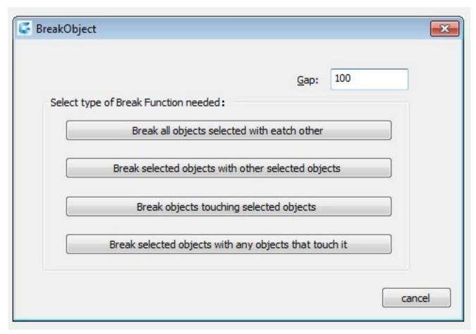
This tool provides four breaking modes with gap distance to visualize the differences between breaking options.
