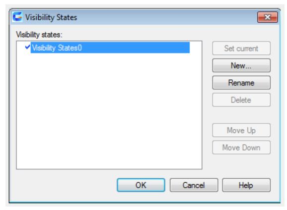
After inserting visibility parameter to block definition, users could edit it in "Visibility States" dialog box.
