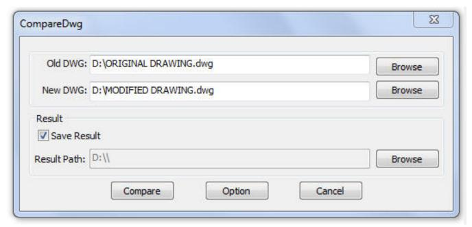
In this window, you have to browse the old DWG (original drawing) and the new DWG (drawing modified). You can also assign a path to save the compared drawing. Then select the button Option to setup the comparison parameters.
