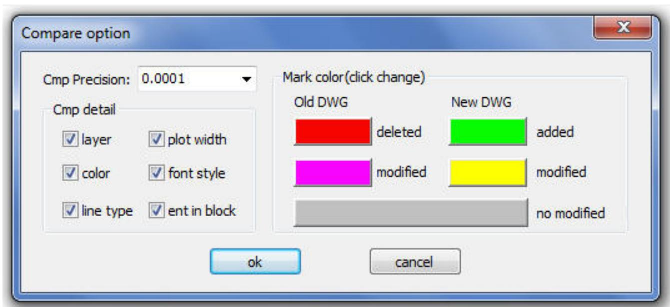
After setting up the comparison parameters such as: colors, layers, line type, etc. select Ok to confirm these parameters. Note: Pay attention to the mark color because the deleted, modified and added objects will assume these into the compared drawing. Then select the button Compare in the window below to compare both drawings.
