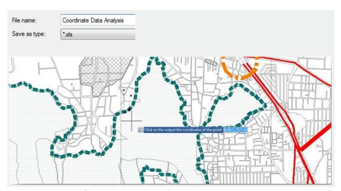
You can open the saved file and check out all coordinate data (X,Y,Z) extracted.
