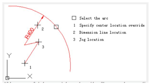
If the center of circle or arc is located outside of layout or does not display its actual position, users could create bending radius dimension for it. Users could specify center location at a convenient position.
