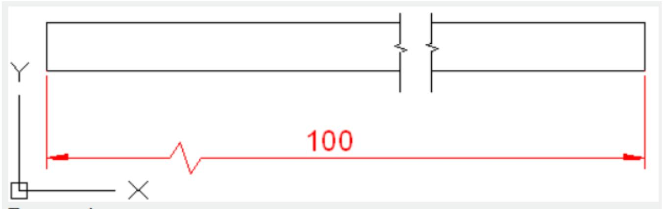
**Remove jog :** Remove a jog from specified linear dimension or aligned dimension.
