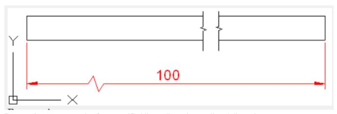
**Remove jog:** Remove a jog from specified linear dimension or aligned dimension.
