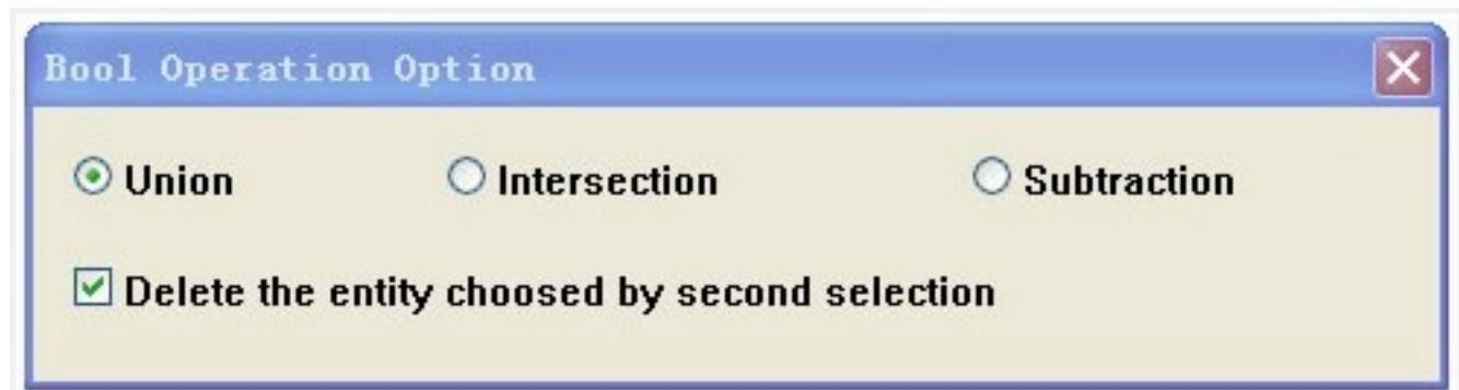
Delete the entity chosen by second selection: Choose whether to delete the second selected object. There are different Boolean operation options such as union, intersection and subtraction. After the operation the object will be a polyline.
