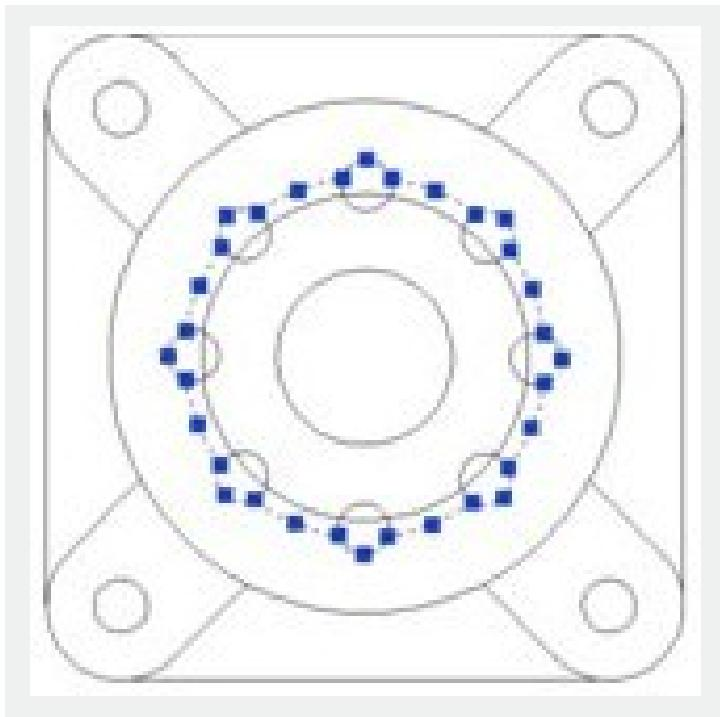
4. Start again the boolean operations, select option "subtraction" and check "Delete the entity chosen by second selection", as shown.
