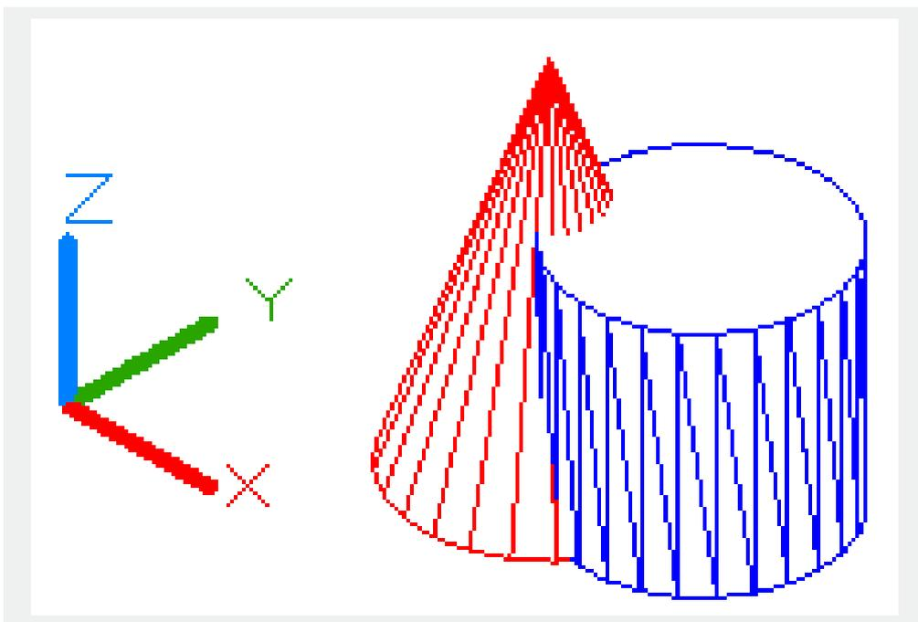
Users could use VPOINT and VIEW commands to create a 3D view for a 2D drawing and display its wireframe. All lines are visible, including lines covered by other objects. The HIDE command could hide those covered lines.
