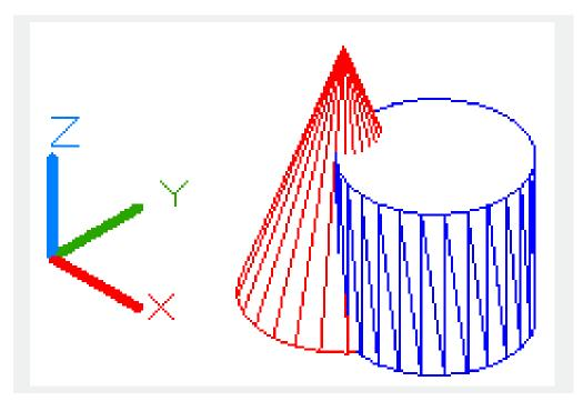
Users could use VPOINT and VIEW commands to create a 3D view for a 2D drawing and display its wireframe. All lines are visible, including lines covered by other objects. The HIDE command could hide those covered lines.
