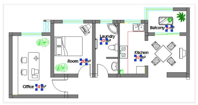
In the Statistics dialog box, you can see the cumulative sum from the selected text numerical values. You can also re-select, replace, copy text numerical value again plus fill-in (show) the cumulative sum in any point of your current drawing
