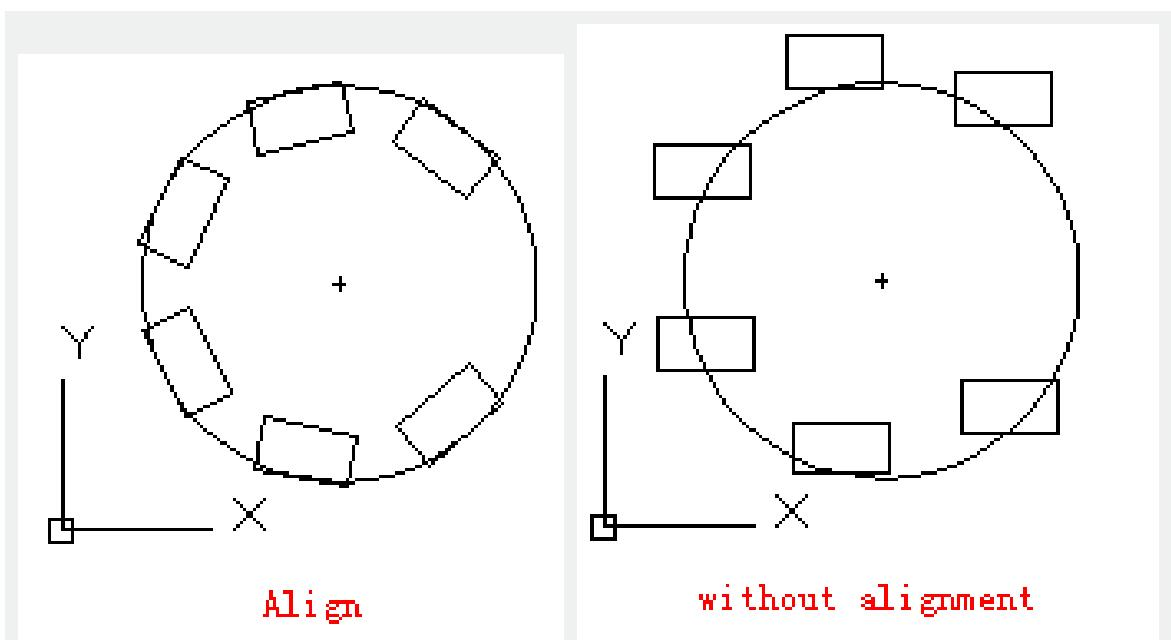
After specifying length of segment, blocks will be inserted by specified interval. If the inserting block containing some variable attributes, those attributes will be abandoned.
