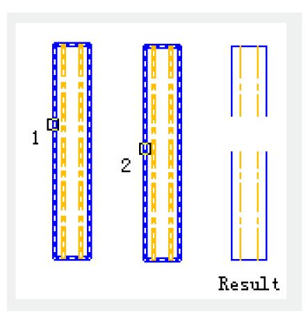
Weld All Weld the broken Mline.
