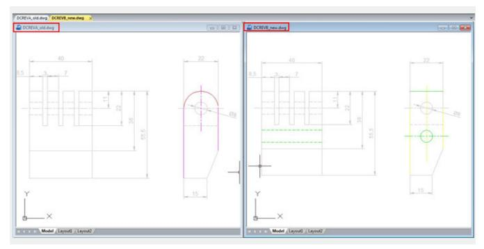
But there is something else that drawing compare could not accomplish so accurately. Drawing compare can't insert and show the compared objects on the current drawing working space that you are working at real time. Besides, drawing compare can't show the details of how the objects were located before they were modified.
