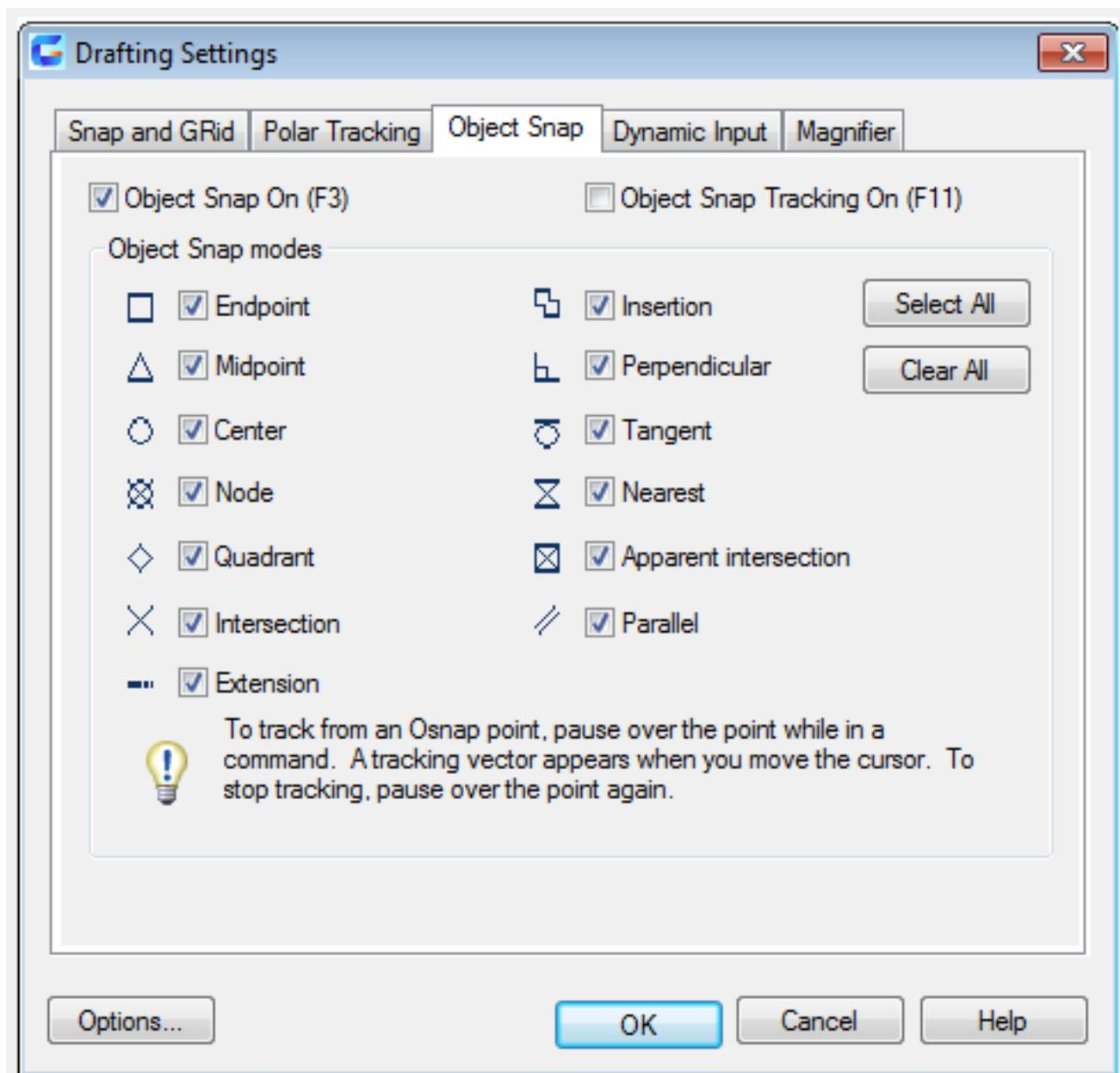
The drafting settings dialog box is used to specify the settings of Snap and Grid, Polar Tracking, Object Snap.
